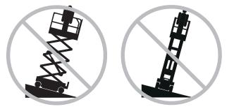
Models with outriggers: Do not lower the outriggers unless the machine is on a firm surface. Avoid drop-offs, holes, unstable or slippery surfaces and other possible hazardous conditions.
